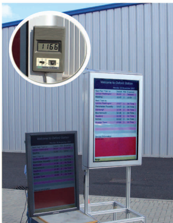
High Brightness Display Compared to standard 450 cd/m 2 display
